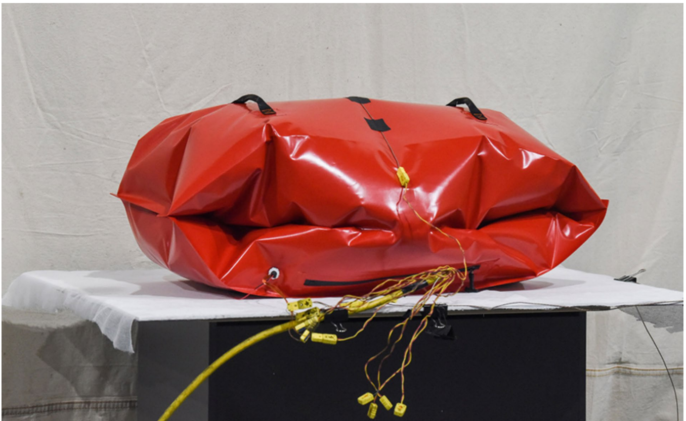
Figure 1: Fire containment product designed to mitigate hazards from lithium-ion battery fires, shown here during testing.
